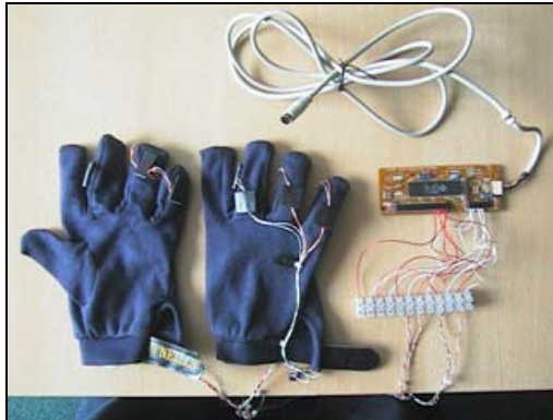
Figure 45. Gloves connected to the keyboard circuit and plugboard.
